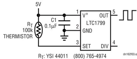
**Figure 3. Temperature-to-Frequency Converter**
