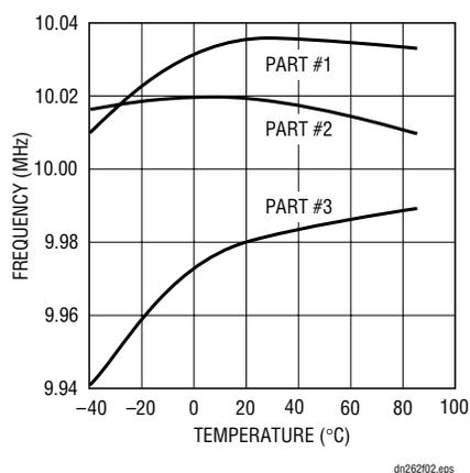
Figure 2. Frequency vs Temperature for Figure 1's Circuit
